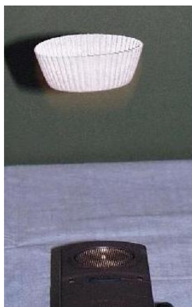
Figure 4. The fall of muffin cups may be studied by using a data logger with a motion sensor.
