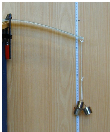
Figure 1. Measuring the displacement of the tip of a clamped ruler as a function of load.
