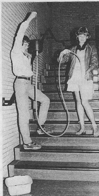
Model of the hose-and-bucket pump without device for raising the bucket
