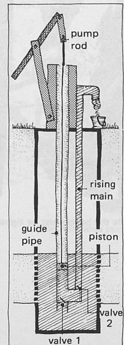
Diagram of the displacement pump
