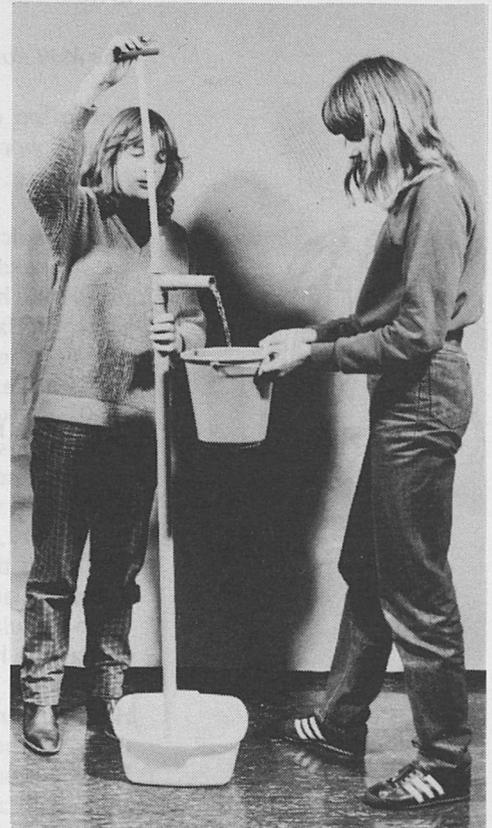
A model of a suction pump made of PVC tubes.
