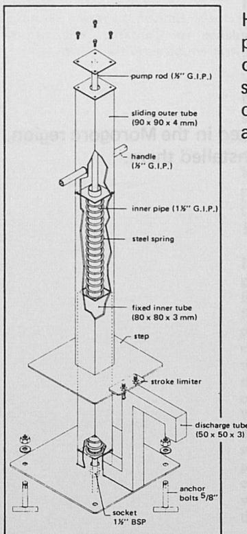
However, the rotating parts of the pump were something of a problem and the pump broke down. A second pump, known as the kangaroo pump, was developed without rotating parts and that worked. When you step onto the pump a spring is depressed and the piston descends. When you step off, the spring is depressed and the piston descends. When you step off, the spring is released and the piston comes up again.
