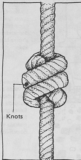
The special knot for the rope pump.
