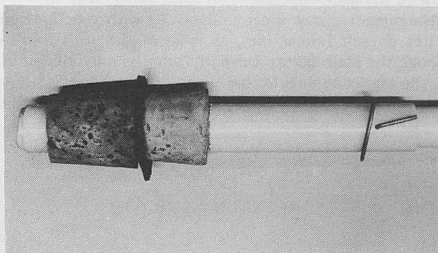
A piston for the suction pump. Note how it differs from the piston of the displacement pump on page 29; the corks are reversed.
