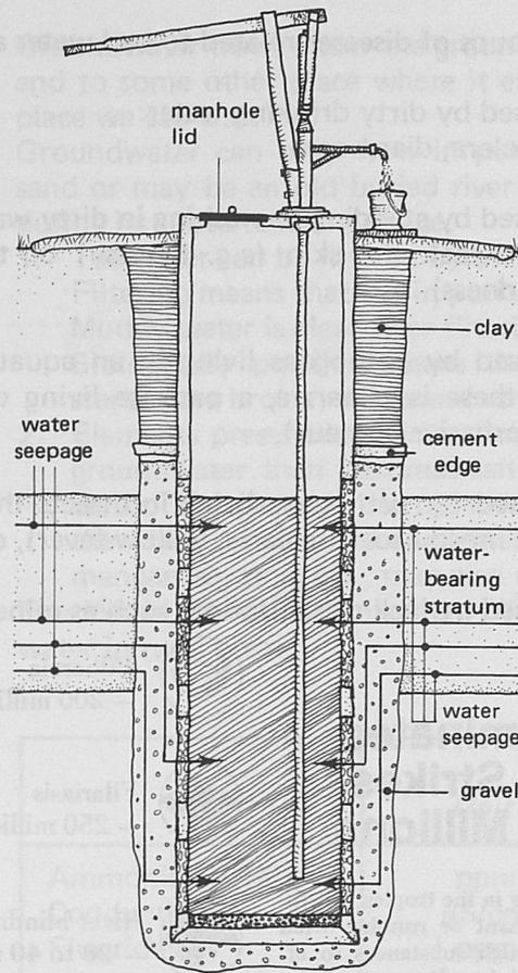
This is how water seeps from the water-bearing stratum into the well
