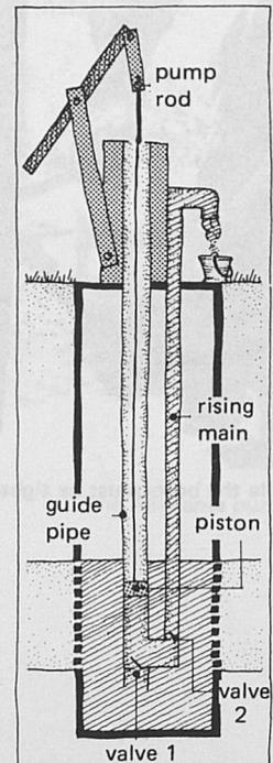
Diagram of the displacement pump
