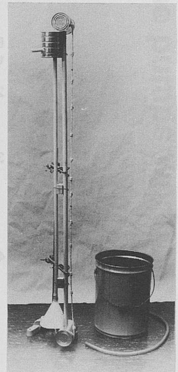
Model of the rope pump without wheel or handle.
