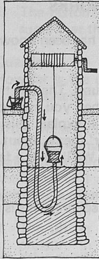
Just as your finger was sucked into the pipe when the bucket was lowered, so will the water be if you leave the end of the hose in a full bucket. The water will be sucked out of the full bucket and into the bucket connected to the hose. This process will continue until the water level in the bucket has dropped to the point where air is being sucked into the pipe. This is known as *siphonage*.
