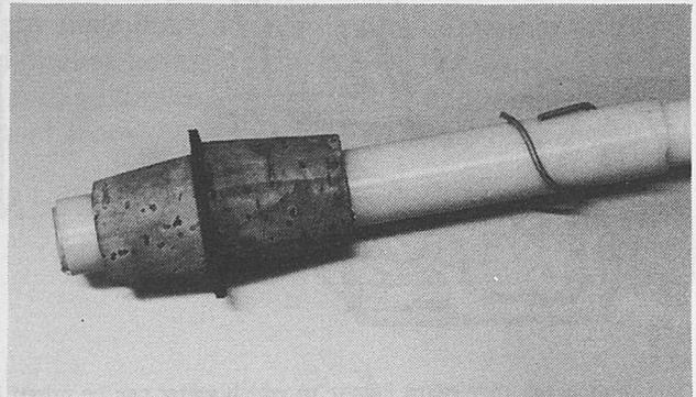
One way of making the piston. Note how the piston differs from that of the suction pump on page 36; the corks are reversed.
