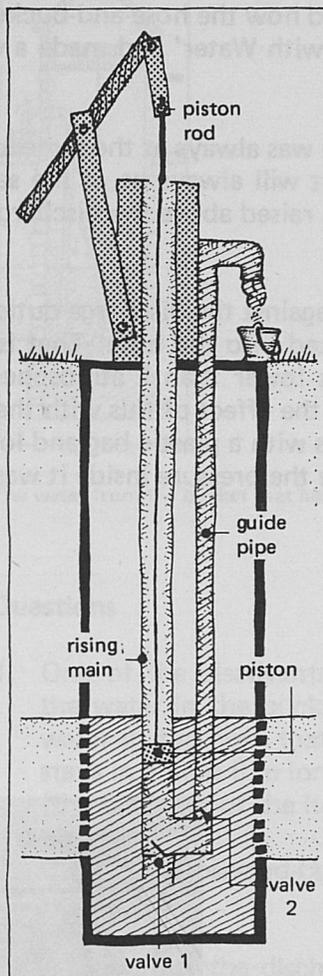
The displacement pump works with a submerged piston. When the piston rises, water flows into the cylinder; when the piston is moved downwards, the water from the cylinder is forced upwards.
