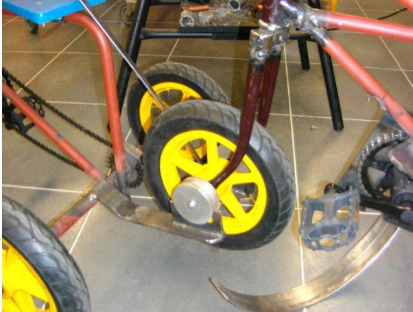
Fig. 5 Connection between bicycles of a two-part detachable tandem at school 4
